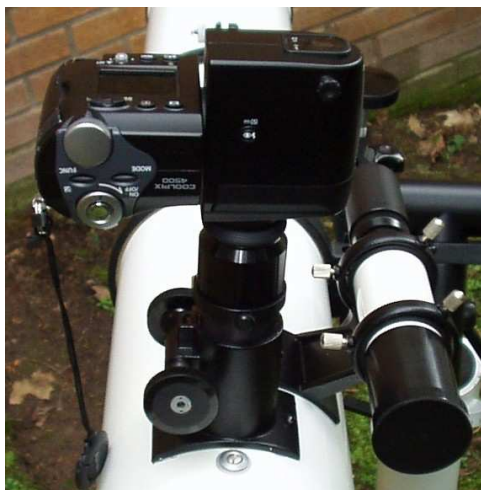
Camera and adapter fitted to telescope
