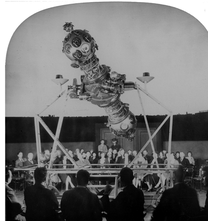
A Zeiss Mark-II Dumbbell Projector
